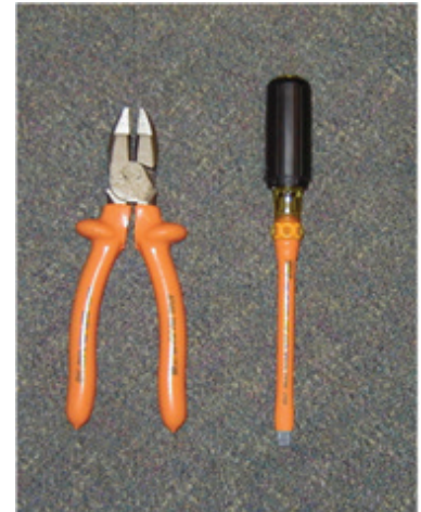
Voltage rated insulated tools
