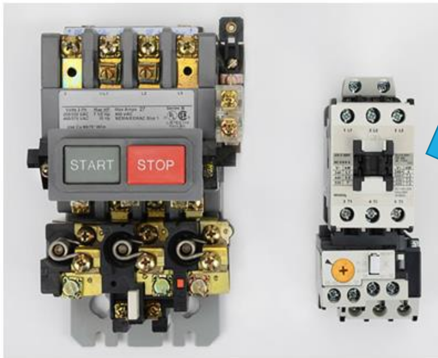
Figure 1. This NEMA starter and IEC starter are each sized for up to a 27-amp load, with the NEMA starter capable of a wider range of duty befitting its larger size and greater weight.
